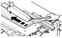
Set the cutting height of the saw blade. The blade guard must rest with its front edge on the workpiece.
